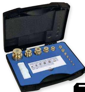
Plastic box, lined, for weight sets, knob shape, stainless steel or finely turned brass
