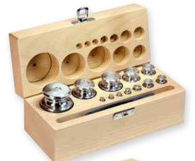
Wooden box, for weight sets, knob shape, stainless steel or finely turned brass
